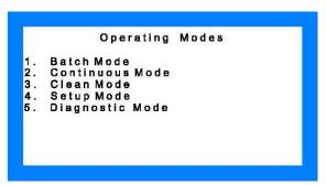
To select one of the modes listed on this screen, the number 1, 2, 3, 4, or 5 must be pushed, followed by the "ENTER" button. When starting the system for the first time, it is best to push "4" and then "ENTER" to go into the Setup Mode. In this mode, the concentration can be changed from the default concentration of 8000 PPM to a different value, if desired. The Power Save option can be turned "OFF"
